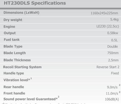
$<sup>^{*1}</sup>$ Vibration Level on the handles measured according to ISO 5349 (m/s )
