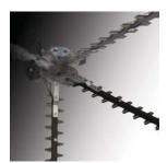
**Articulated Blade**The AHT235D series features an articulated blade which can rotate 132°.
