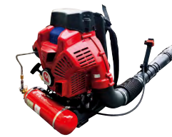
Blower prototype using hydrogen engine
